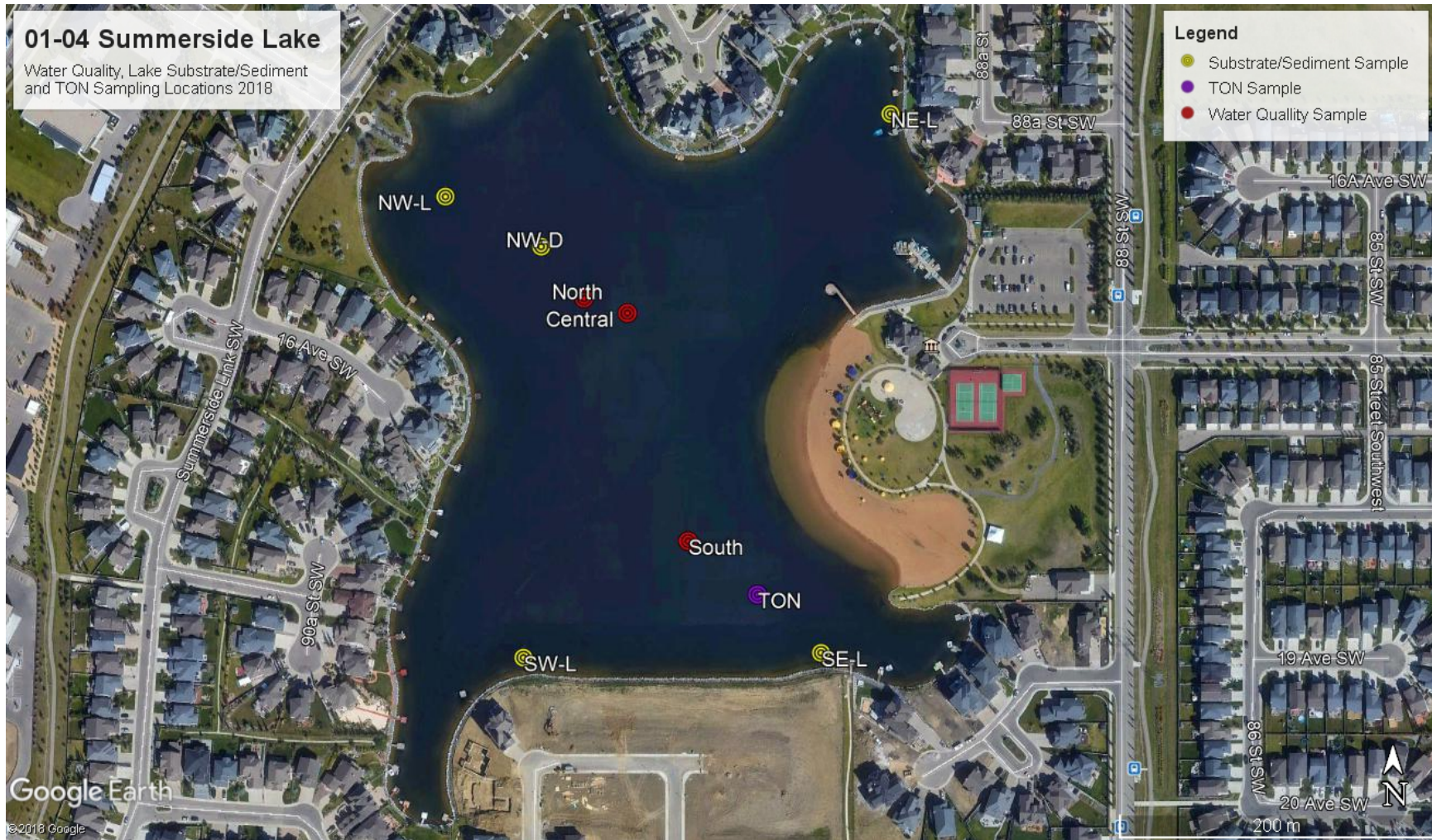
Figure 9.1. Water quality, substrate/sediment and threshold odour number (TON) sampling locations in Summerside Lake. Water quality samples collected on various dates in 2018; substrate/sediment samples collected August 14, 2018.
