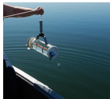
Figure 2. Horizontal Beta bottle with collected sample.
